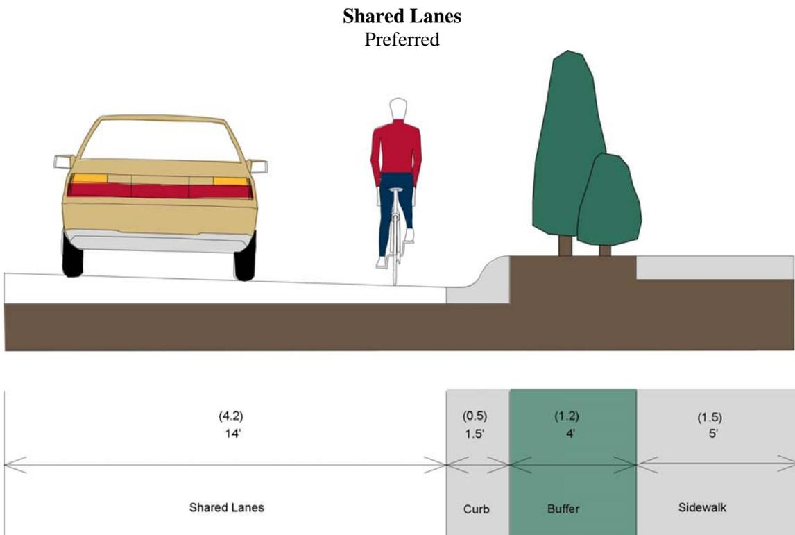
Shoulders: Shoulders must be paved and a minimum of 4 ft (1.2 m) wide when they are designed to accommodate bicycle travel. A width of 5ft (1.5 m) or greater is preferable and additional widths are desirable where substantial truck traffic is present, or where motor vehicle speeds exceed 50 mph (80 km/h).
