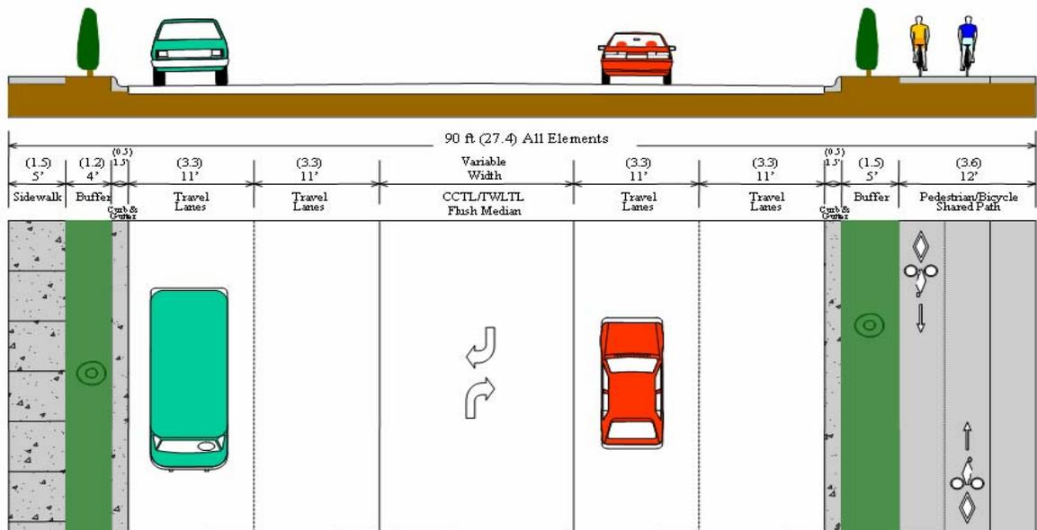
**CLASS IV Minor Arterials** provide network connections within and through the urbanized area. These facilities typically provide a greater amount of access to adjoining land as compared to principal arterials.
